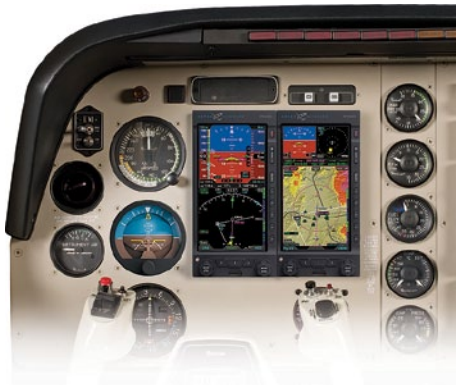
Figure 1-3 Dual Display System: PFD & MFD
