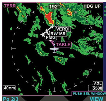
Figure 2-3 Dedicated Terrain Display on the EFD1000/500 MFD
