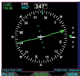
Figure 5-90 Secondary HSI Displaying the VDI
