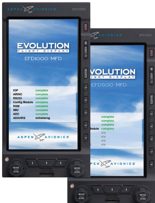
Figure 4-1 EFD1000/500 MFD Initializing Screen
