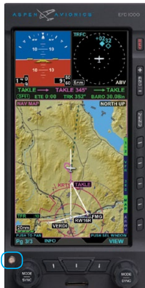
Figure 4-26 EFD1000/500 MFD photocell
